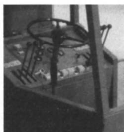
Full instrumentation is located in the operator's compartment for travel, steering, hoisting, sling spacing and load controls.
