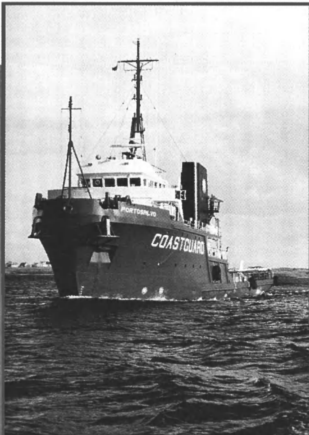
British standby vessel Portosalvo features a bollard pull of 147 tons.
