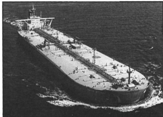
Navix Astral from Hitachi Zosen is a 259,987-dwt, 1,062.6-ft. (323.9-m) long VLCC delivered to Golden Bayshore Corp.
