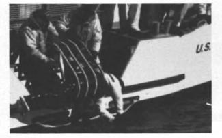
JASON'S CRADLE forms a par-buckle, giving the rescuer a 2:1 mechanical advantage. In most situations, once the casualty is placed in the non-collapsible loop, the recovery process takes 4-8 seconds
