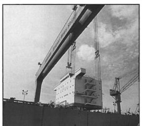
Pictured is the installation of the deckhouse on Double Eagle tanker Despotico at Newport News Shipbuilding.
