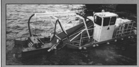
This "combo" oil/debris Marineskimmer offers rapid response to typical non-catastrophic, protected water oil spills commonplace in harbors, rivers and navigable waterways.
