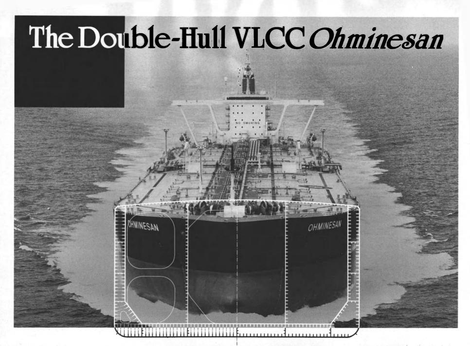
The *Ohminesan* is the fourth double-hull VLCC built by Hitachi Zosen. This new vessel is double-sided and double-bottomed,
