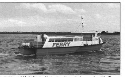
Dickensian vessel Martin Chuzzlewit is now in service on the lower reaches of the Thames. Its long, slender displacement triple hull form provides a wider deck platform than could be accommodated on a monohull, with additional stability.
