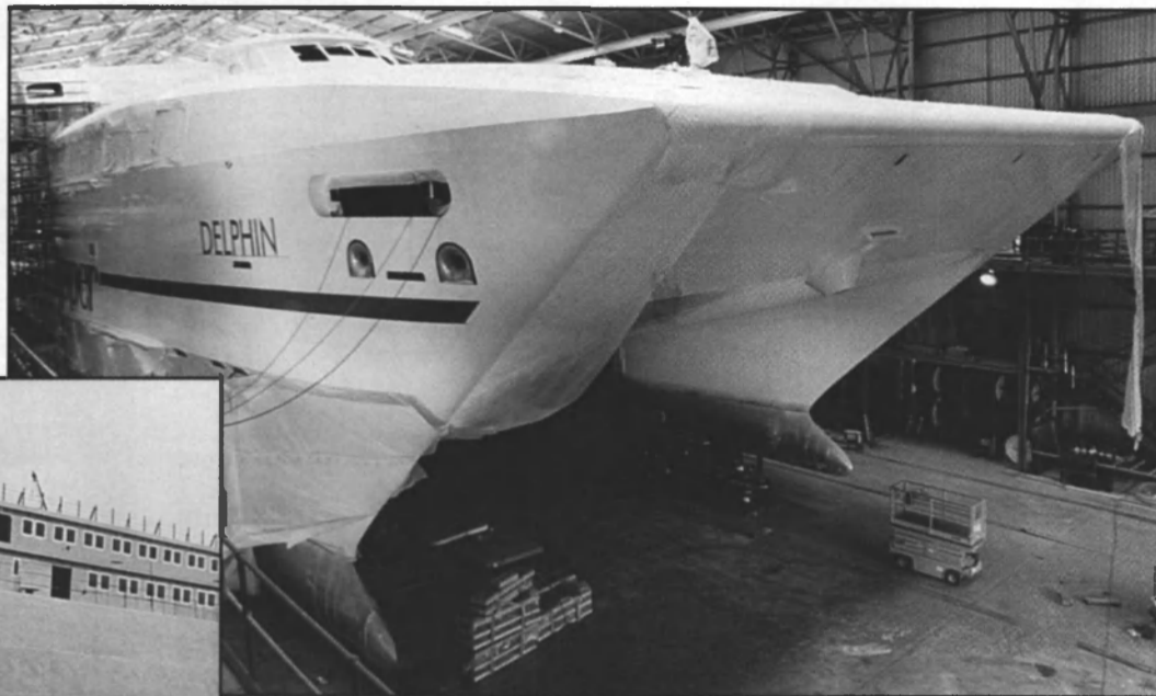
Delphin (above) is scheduled to leave for the Baltic this month to serve on the Rostock, Germany, to Trelleborg, Sweden, route for TT-Line GmbH. Four 600-kW MTU diesels each driving a KaMeWa waterjet will give the vessel a 36-knot service speed when carrying 600 passengers and 175 cars.
