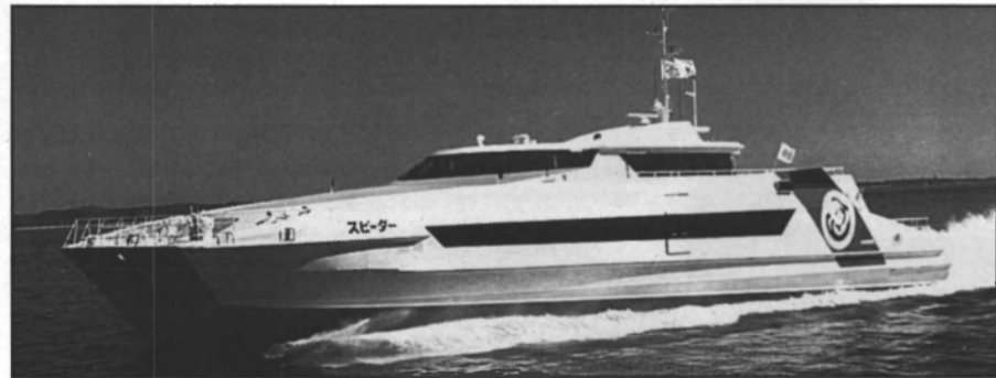
The Ocean Leveller system is fitted to the 43-m Speeder, a passenger catamaran operating in Japan. Fins are located on the in-board side of each hull forward. The stabilizing system has also been installed on TT-Line's Delphin.
