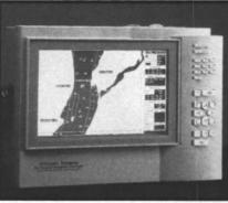
The NAVIGATOR is built to the following MIL-SPEC Specifications: Water resistance & salt exposure; MIL-T 28800c para 4.5 6.2. Vibration 1.5g 10-100HZ Shock 5G peak.
