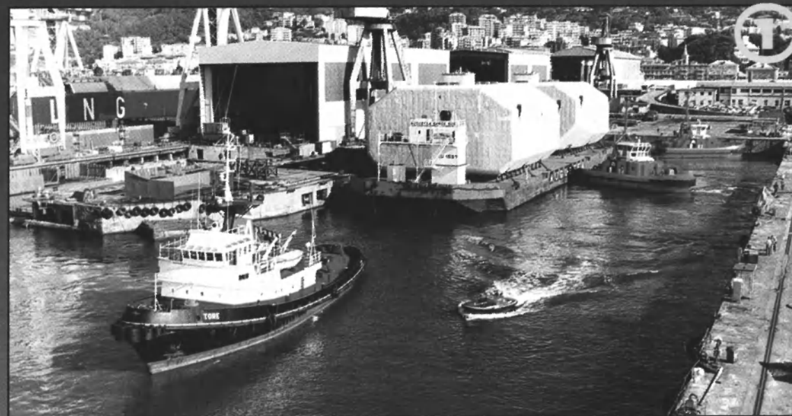
ONE, TWO, THREE: Pictured is the progressive loading of LPG tanks into the newbuilding LPG carrier Sestri Cantiere Navale is building for Carbocoke. Each tank weighs 700 tons. The newbuild can be seen right alongside another newbuilding, Snam Portovenere , an LNG carrier.
