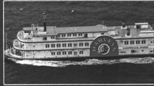
KANESVILLE QUEEN - 272' x 72' built for Harveys Casino Resorts for service in Council Bluffs, Iowa on the Missouri River. Two full decks and a partial third deck will provide 30,000 sq. ft. of casino area for 1700 passengers.
