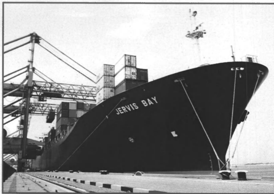
The IHI-built Jervis Bay , one of a series of seven 4,236-TEU containerships built for P&O Containers, features Marlow Steeltite H.M.P.E. mooring ropes, which reportedly exhibit the strength and extension of conventional steel wire rope while being only one-sixth the weight of a wire rope of equal strength.
