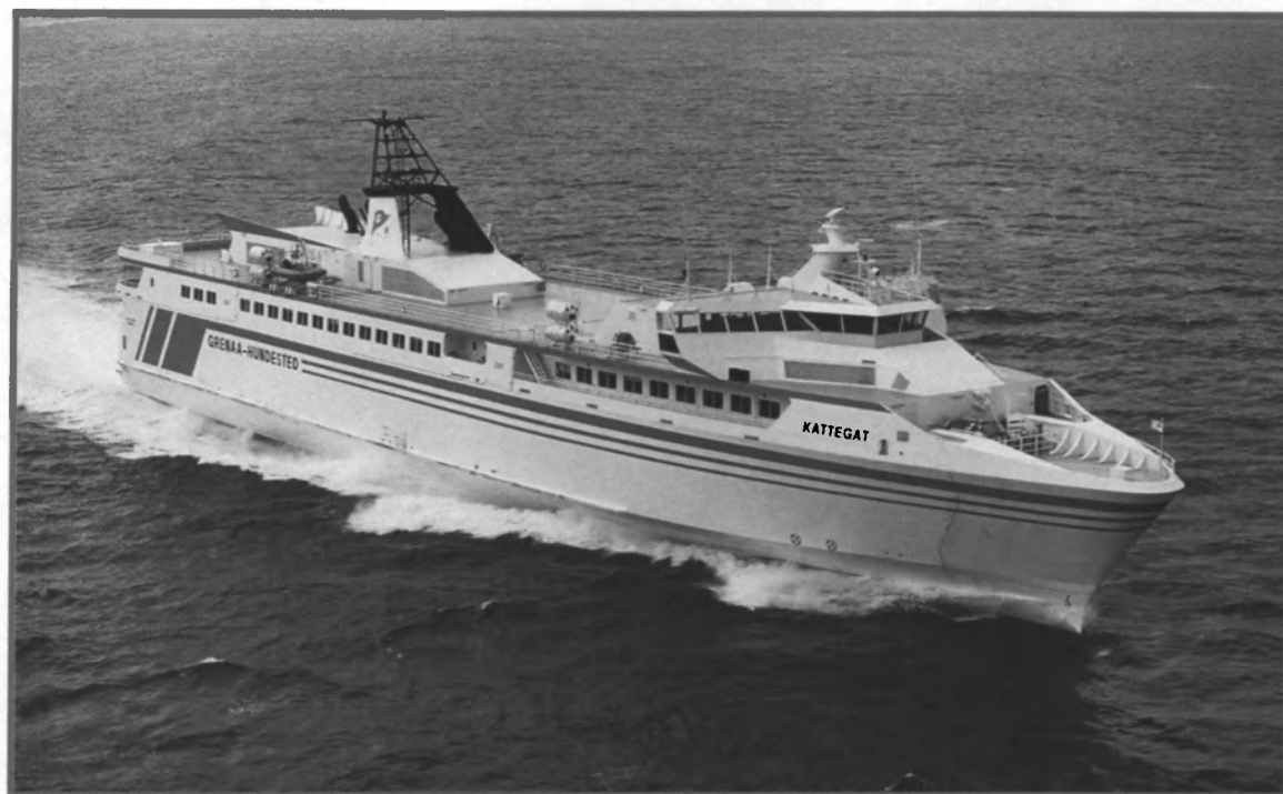
LEFT: The Kattegat , powered by four 20-cylinder series 1162 MTU engines, recently entered service. ABOVE: Austal Ships will build a 270-ft. (82.3-m) ferry for German operator TT Line, powered by four 20V 1163 MTUs. BELOW: Each Elbe City Jet — reportedly the first catamaran ferries to operate on the Elbe — will have two 8V 396 engines from MTU. A spare will be kept at the MTU Product Support Center in Hamburg to ensure adherence to the vessels' rigorous schedules.
