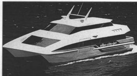
LEFT: The Kattegat , powered by four 20-cylinder series 1162 MTU engines, recently entered service. ABOVE: Austal Ships will build a 270-ft. (82.3-m) ferry for German operator TT Line, powered by four 20V 1163 MTUs. BELOW: Each Elbe City Jet — reportedly the first catamaran ferries to operate on the Elbe — will have two 8V 396 engines from MTU. A spare will be kept at the MTU Product Support Center in Hamburg to ensure adherence to the vessels' rigorous schedules.
