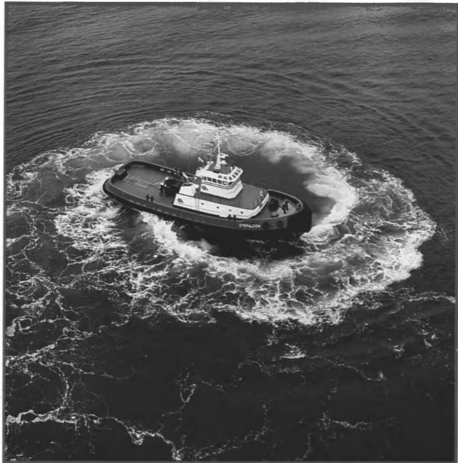
Z-Drive-Equipped Gyrfalcon Spins Out: As reported in MR/EN's October edition, Marco Seattle's latest workboat newbuild, Gyrfalcon, is equipped with features that conform to a recent workboat propulsion trend — Z-drives — driven by twin diesels, Caterpillar 3516 B Series diesels, each rated at 2,000 bhp.
