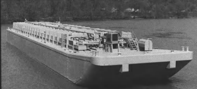
200 Foot, 10,000 BBL Tank Barge
