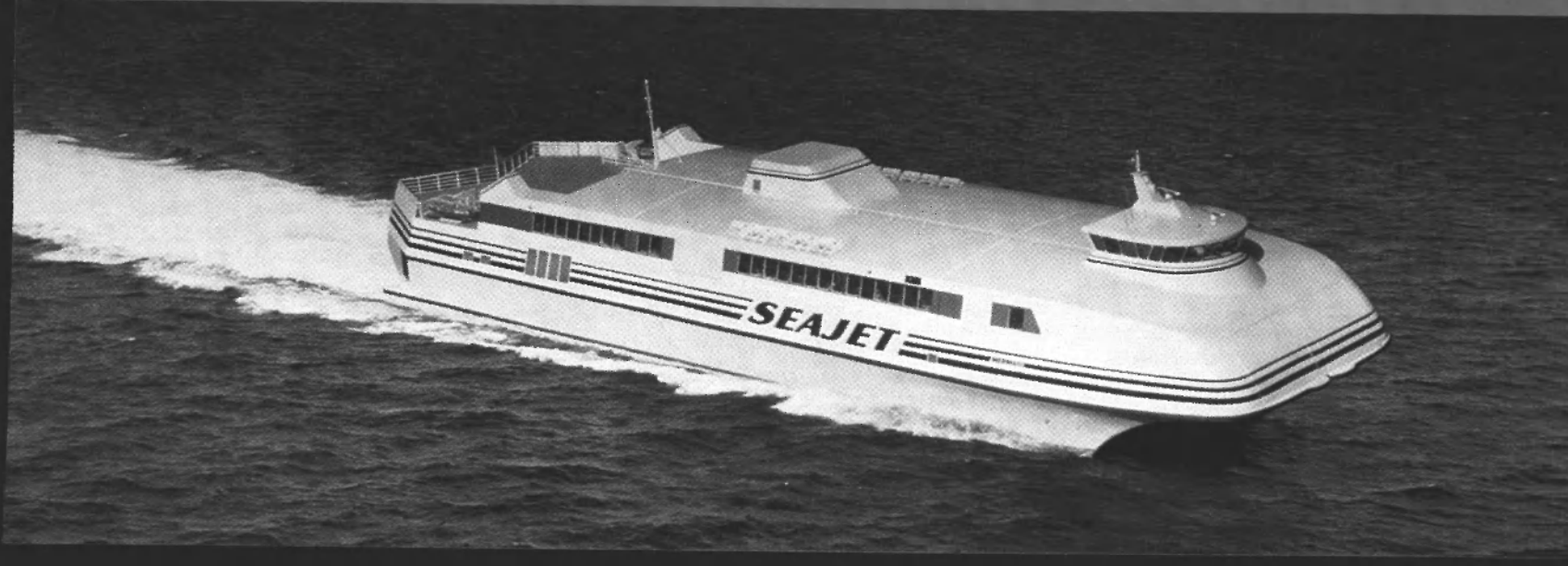
GE LM1600 gas turbines will power two SeaJet passenger/car fast ferries for Danish operator Mols-Linien. The vessel was designed by Danyard A/S in conjunction with NQEA of Australia. (See page 64).
