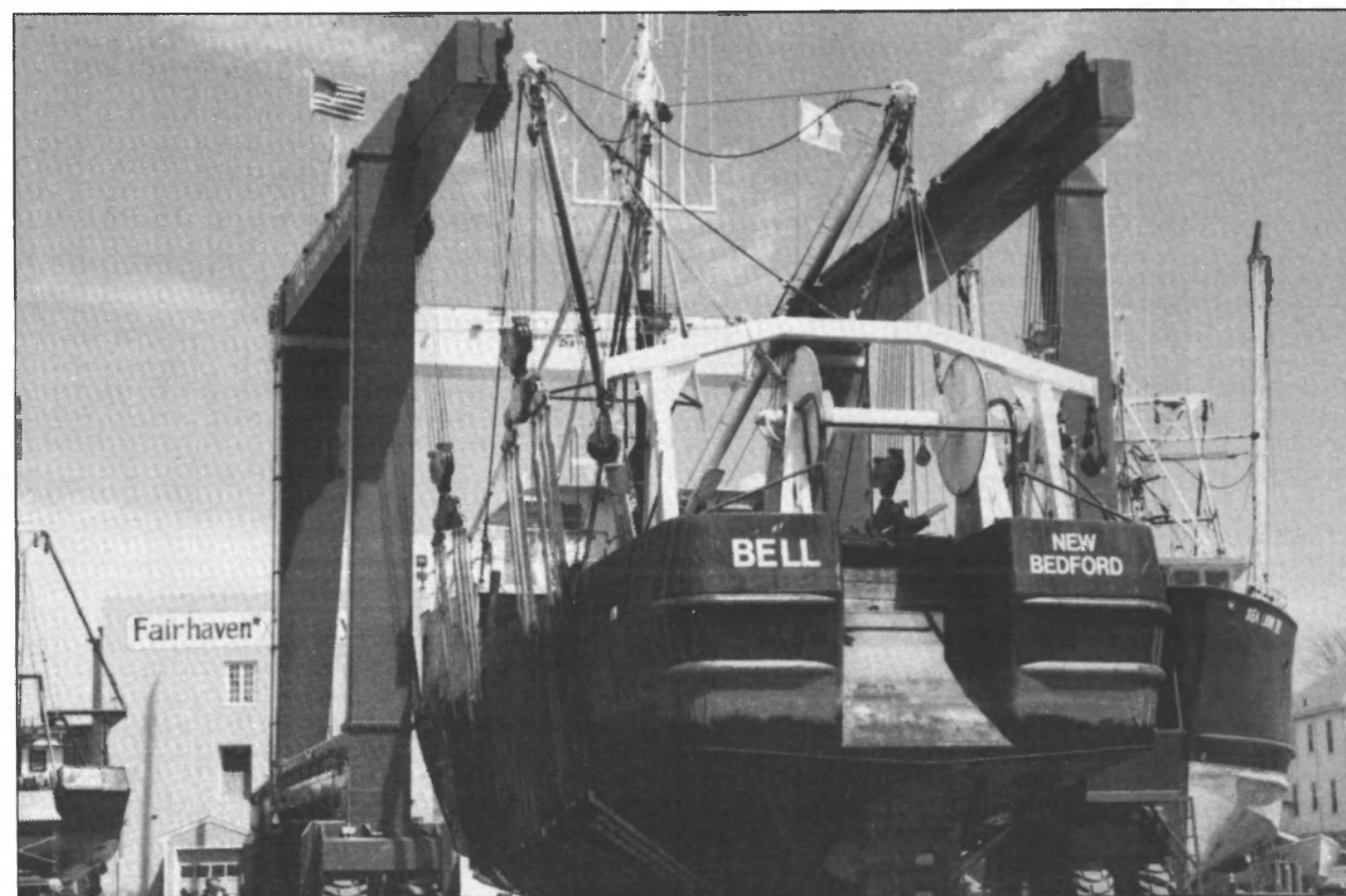
A model 300 BFM mobile hoist rated at 600,000 lbs. shown at Fairhaven Shipyard, Fairhaven, MA.
