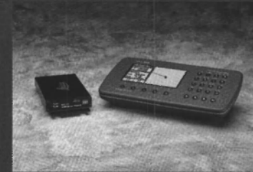
The MX 100 GPS Navigator combined with the MX 41R Beacon Receiver provides accuracy to under 5m.
