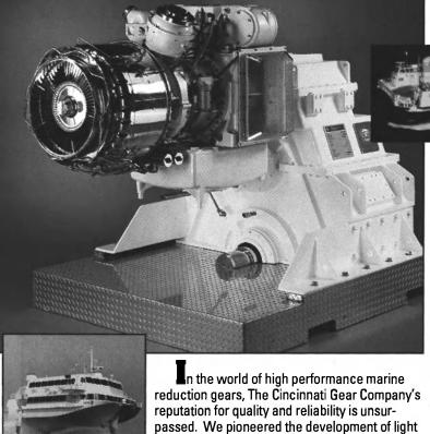
passed. We pioneered the development of light weight gas turbine marine reduction gears in the early 1970's with the design and production of the marine gear for the Kawasaki/Jetfoil high speed passenger ferry. Today over 40 of the Jetfoil crafts and 110 gearboxes have been produced, logging well over 600,000 hours of trouble free operation.
