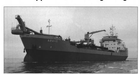
Hopper suction dredger Aru II is one of two nearly identical vessels delivered to a state-owned Indonesian enterprise by Krupp Fordertechnik. A cutterhead suction dredger, Batang Anai, is scheduled for delivery to the same customer this fall.
