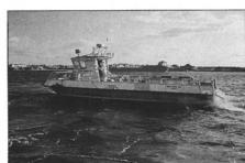
The first Marshall Branson Marine (MBM) boom deployment vessel, specifically designed and constructed to meet the requirements for rapid response to oil spillage incidents requiring immediate containment and removal, was delivered for operation in South Korea.
