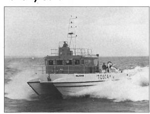
Twin Volvo Penta TAMD 122D turbocharged and aftercooled diesels provide the propulsion power for Recover. Recover is the Protector 54based oil spill recovery vessel (OSRV) completed by Prout Catamarans for Thames Oil Spill Clear-ance Association (TOSCA), and operated on its behalf by the Port of London Authority (PLA).
