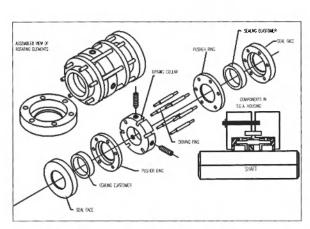
Mechanical drive mechanism for S.E.A.-Seals.
