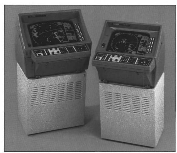
PATHFINDER/ST ARPA: 34-cm or 25-cm PPIs (16" or 12" diagonal CRT IMO equivalents) provide automatic tracking of up to 40 targets with vectors and readouts for the most dangerous 20. Have auto and manual acquisition, and unique trial
