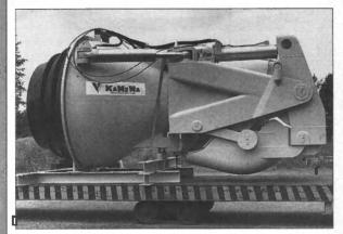
Four KaMeWa size 160 waterjet units are being installed in Stena's high-speed sea service ferry. With an output of 16,354 kW each, these units are reportedly the most powerful waterjets with steering and reversing gear built in the world to date.
