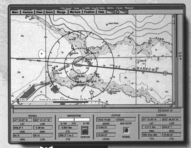
incorporates over 100 navigational functions including route planning and monitoring, multiple hazard alarms, chart updating, voyage recording & replay, range & bearing calculations, vector object overlays, target tracking, and much more. The vessel's position, course and speed information ( from LORAN, GPS or DGPS ) is updated every second and overlaid on the digital chart. The full colour digital charts give you the "look and feel" of traditional paper charts.
