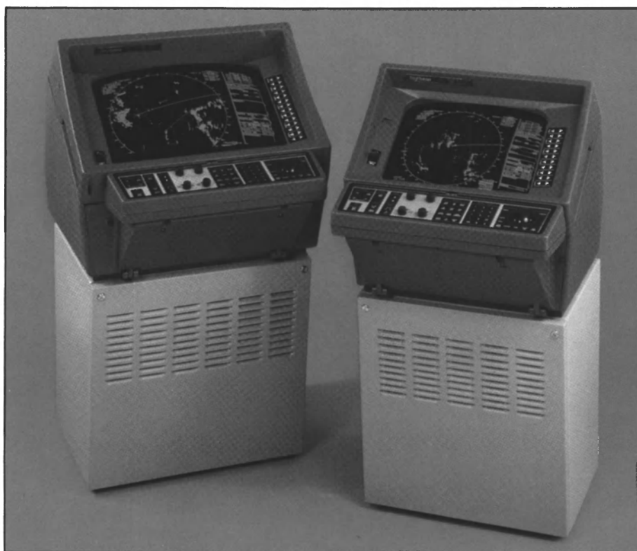
PATHFINDER/ST ARPA: 34-cm or 25-cm PPIs (16" or 12" diagonal CRT IMO equivalents) provide automatic tracking of up to 40 targets with vectors and readouts for the most dangerous 20. Have auto and manual acquisition, and unique trial maneuvers.
