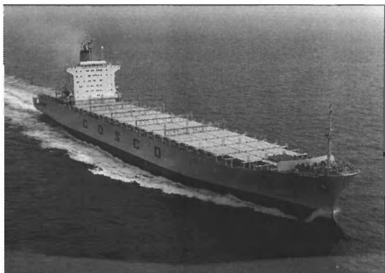
The Da He features a Hitachi Zosen-Sulzer diesel engine, which powers drive the 3,800-TEU containership to a service speed of 24 knots.
