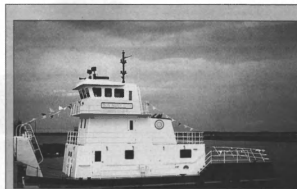
Sun State Marine, Inc., Green Cove Springs, Fla. completed construction of a new towboat which was christened Sun River City . The 1,000-hp towboat is powered by two Caterpillar 3412DITA engines driving MG 521 reduction gears. The main engines were provided by Ring Power Corp. of Jacksonville, Fla. Main and auxiliary electrical power is furnished by two Perkins 40-kW generators. The design drawings were provided by Rodney E. Lay & Associates.
