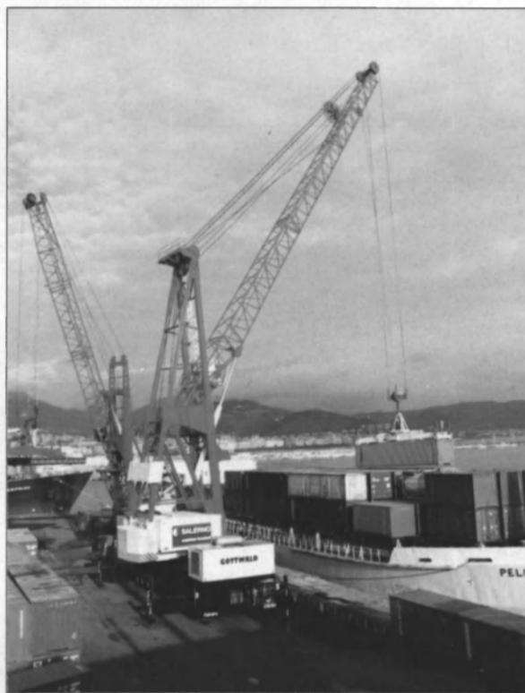
HMK 280 mobile harbor crane from Mannesmann Demag Gottwald employed in container transshipment operations at the port of Salerno, Italy.
