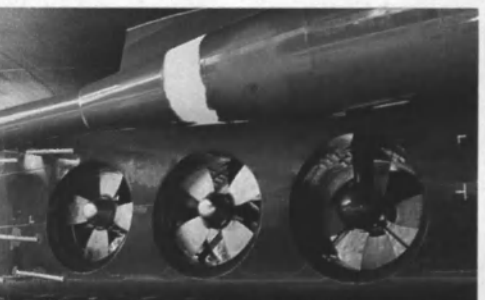
3 x 1500 KW STERN THRUSTERS TYPE: BRUNVOLL SPA-VP
