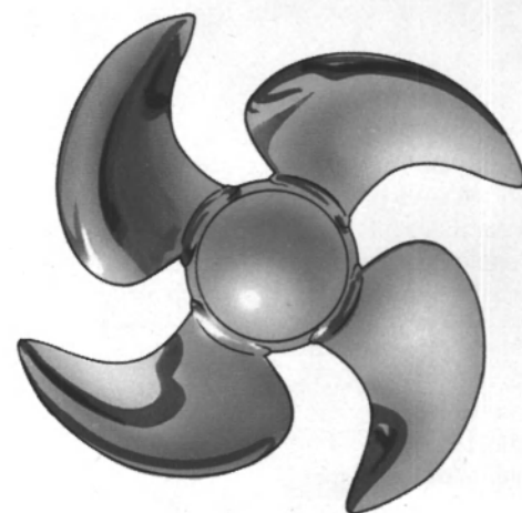
Propeller for car-passenger ferry. High-skew blade shape for low noise and minimized vibrations. (5.1 m diameter, 15640 kW, 23.2 knots)
