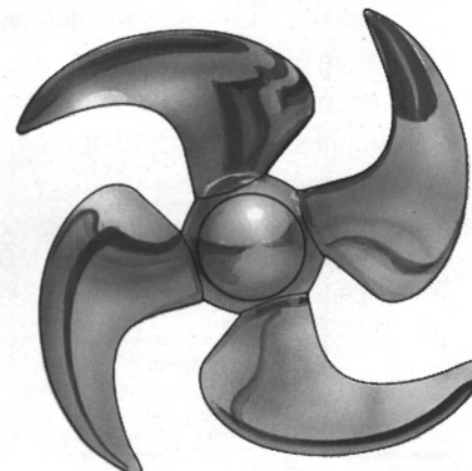
Propeller for cruise ship. High-skew type for low noise and vibration level. (5.2 m diameter, 11820 kW, 22.6 knots)
