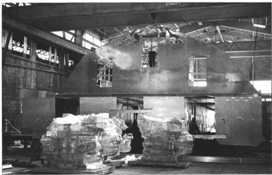
Caterpillar diesel engines sit shrink-wrapped in back of the first Quadrimaran vessel to be built for a commercial customer at the Quadrimaran facility in France.
