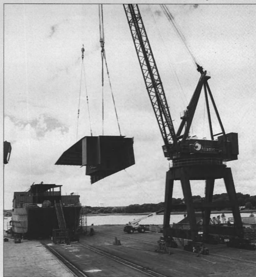
A 150-foot gantry crane sets the forward section of the superstructure on the gaming vessel Empress II, built at Atlantic Marine.
