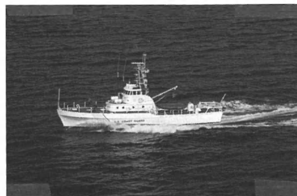
One of the 26 USCG 82-foot patrol boats re-engined with Caterpillar V-12 diesels.
