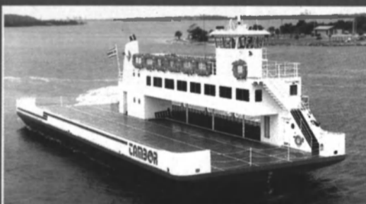
TAMBOR — 130' x 45' double-ended passenger/vehicle ferry. The Tambor is operating between Putarenas and Tambor in Costa Rica.
