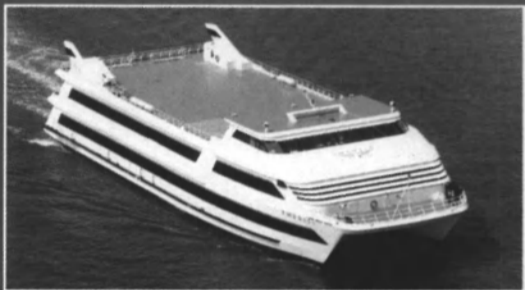
EMPRESS — 222' x 66' ultra modern gaming vessel built for Des Plaines River Entertainment Corporation, Joliet, Illinois. Two ballroom-size casinos on the upper and lower decks provide comfort and enjoyment for the 1200 passengers.
