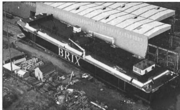
The double-hull petroleum barge "Cascade," built by Zidell and leased to Brix Marine.
