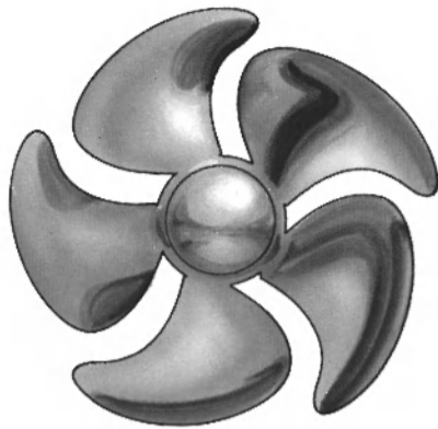
High-skew propeller for frigate, designed for silent operation. (4.2 m diameter, 19180 kW, 31.6 knots)
