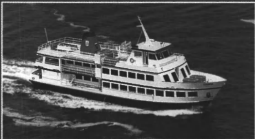
CANIMA — 116' 6" x 31' passenger tender built for the Government of Bermuda with a capacity of 750 passengers to serve the Port of Hamilton, Bermuda.
