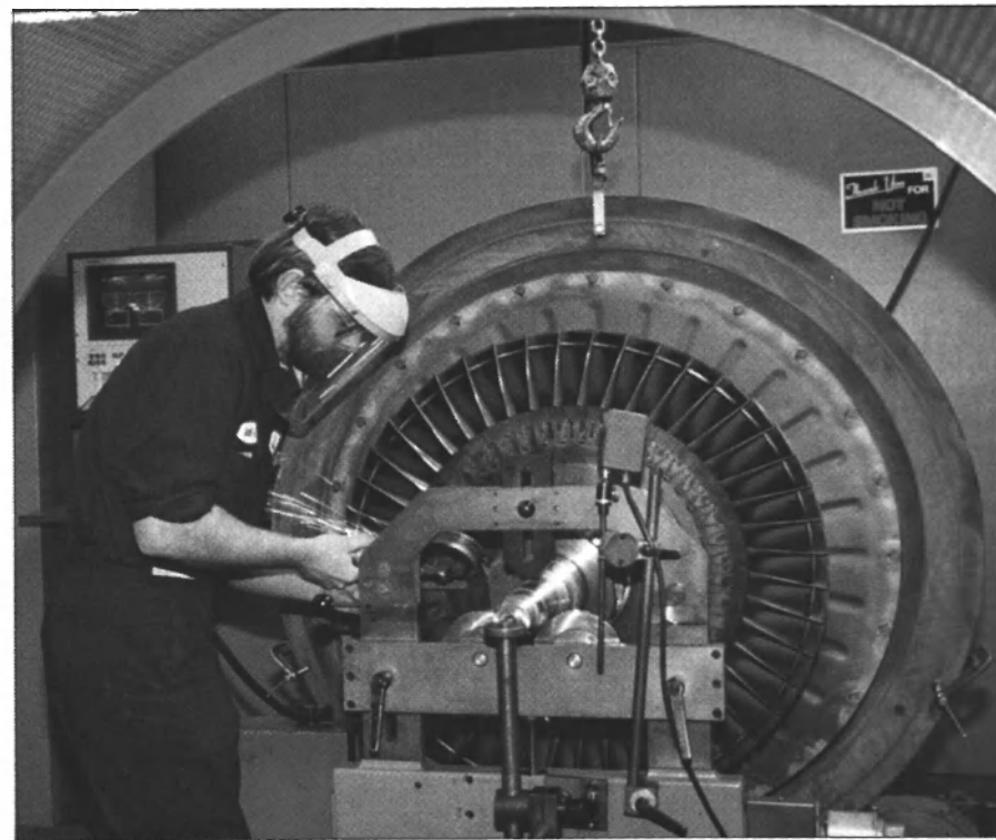
Balancing of a VTR714 Turbocharger Rotor
