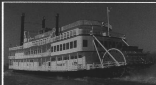
DIAMOND LADY — 201' x 46' Sternwheel Casino Vessel built for Steamboat River Cruise Lines, Bettendorf, Iowa. This 1200 passenger casino vessel, along with her sistership Emerald Lady, provides gaming entertainment in Biloxi, Mississippi.
