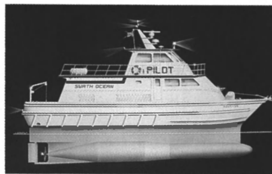
SWATH vessel: "Chubasco" built by SWATH OCEAN SYSTEMS Stats: 72 ft. / 31 ft. beam / 70 tons
