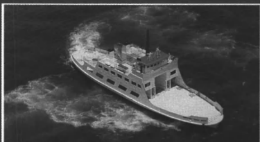
MARGARET CHASE SMITH — 166' x 40' double ended ferry boat with a capacity of 226 passengers and 30 autos built for the State of Maine, for transportation between Isleboro and Lincolnville, Maine.
