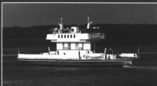
WILLIAMSBURG — 200' x 64' ferry built for the Commonwealth of Virginia carries up to 55 vehicles and 350 passengers.
