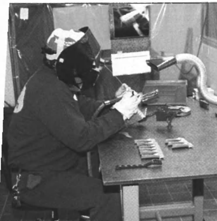
Reconditioning/welding of turbocharger blades in a specially designed, clean and climate-controlled room.
