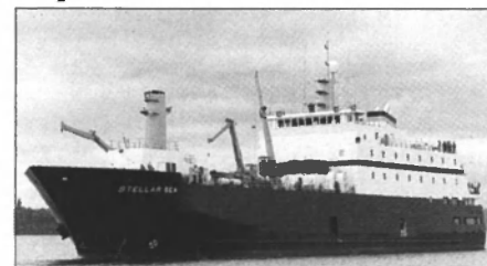
Ak-Wa, Inc. transformed a container ship into this seafood processor.
