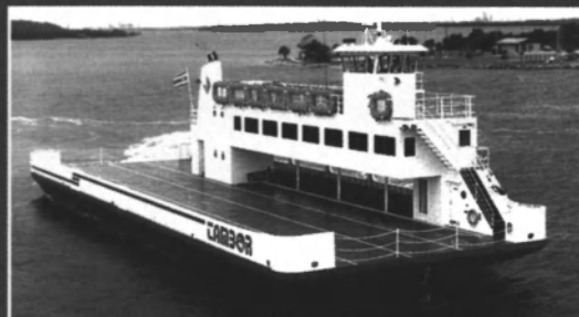
TAMBOR — 130' x 45' double-ended passenger/vehicles. The Tambor is operating between Putarenas and Tambor in Costa Rica.
