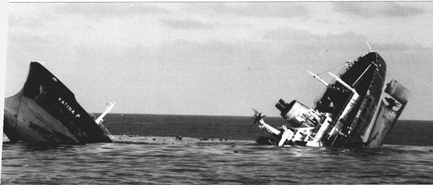
The Polembros Shipping-owned Katina P, a 70,000-dwt tanker, broke her keel during a storm and sank off the coast of Mozambique earlier last year. Salvors helped prevent any major spill.
