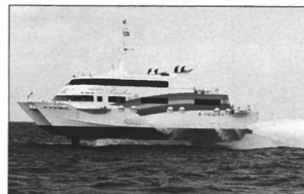
MHI's 'Rainbow,' reportedly the first high-speed, diesel-powered, submerged hydrofoil catamaran.
