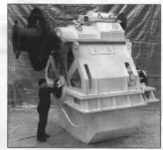
One of the reduction gears being built by Schelde Gears Vlissingen for two containerships.
