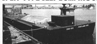
Length . . . . . . . . . . . . . . . . . 180'0" Depth of Mid-Body ..... 14'0" DWT @ d = 10.22 ft. . . . . . 1,615 L.T. Rake Lengths F. & A. . . . . 26'0" Engine GM 671
