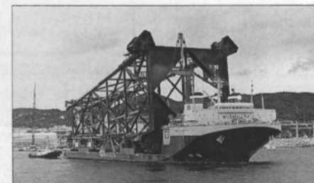
BP's riser jacket loaded aboard the Mighty Servant 2.
