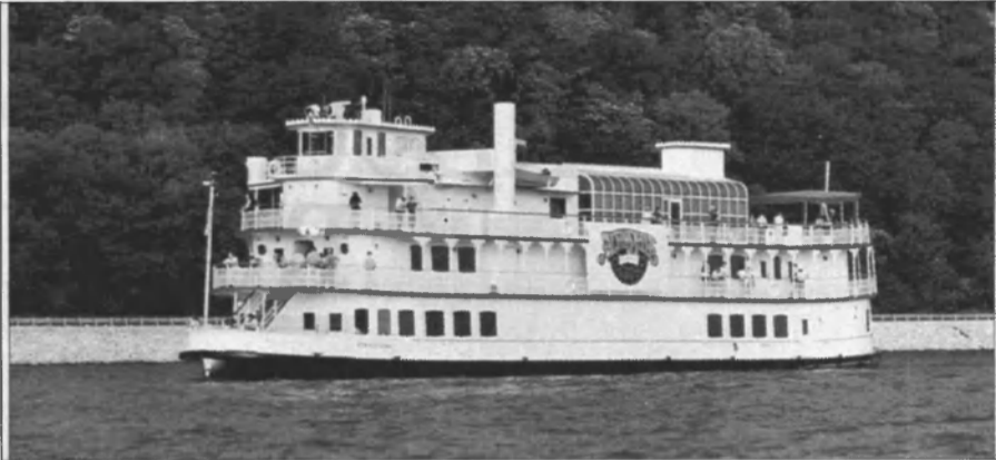
ALTON BELLE CASINO Dimensions: 156 x 34 Capacity: 600 Main engines: Cummins
