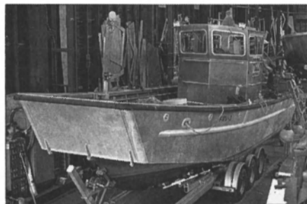
One of the Foss spill response vessels with retrofitted pilot house from Kvichak Marine.
