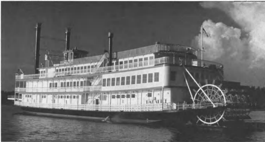
PAR-A-DICE Dimensions: 227 x 46 Capacity: 1,068 Main engines: Caterpillar
