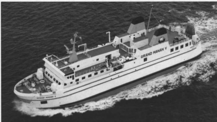
The 246-foot twin-screw ferry Grand Manan V was built by Conoship Contracting for the Ministry of Transportation of the Province of New Brunswick, Canada.
