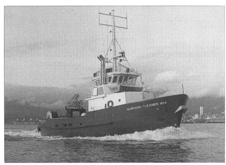
The 75-foot Burrard Cleaner No. 9, designed by MARCO Pollution Control of Seattle, is the largest oil spill recovery vessel serving Canada.
