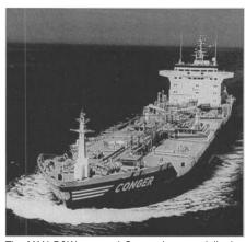
The MAN B&W-powered Conger has specially developed ship lines for an optimized speed/power characteristic and good seakeeping properties. Her Jastram-Werke bow thruster improves maneuverability, while her double bottom and double side shell lower the risk of environmental pollution.
