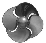
Tunnel thruster propeller with high-skew blades for silent operation. (1.1-3.3 m diameter, 310-3500 kW)
