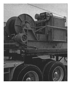
Winches by McElroy Machine to be delivered to U.S. Navy for installation aboard Navy tugs.
