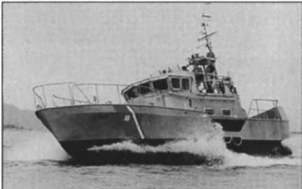
The U.S. Coast Guard's 47-foot motor lifeboat has a maximum operating speed of 28 knots and an associated range of 220 nautical miles. The hull is lightweight yet strong enough to withstand hurricane force winds and 20-foot breaking waves. The boat has the capability of a complete rollover and can self-right in 30 seconds or less.
