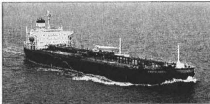
The HZ/MAN B&W-powered product carrier Kastelorizo, built by Hitachi Zosen, has no projections within the tank, thereby shortening cargo-loading time and facilitating tank cleaning.
