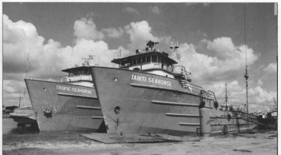
**SEAHORSE CONVERSION**—Besides building the Spirit of Norfolk, Service Marine also has three 176-foot supply oilfield vessels under repair and conversion. The ex-Tahiti Seahorse, soon to be the F/V Arctic Quest, will be converted for Arctic Quest, Inc., Homer, Alaska, and will join the crab fishing fleet near Dutch Harbor. The vessel will feature complete equipment renovation and a new Caterpillar engine and generator package furnished by N.C. Power Systems of Seattle.
