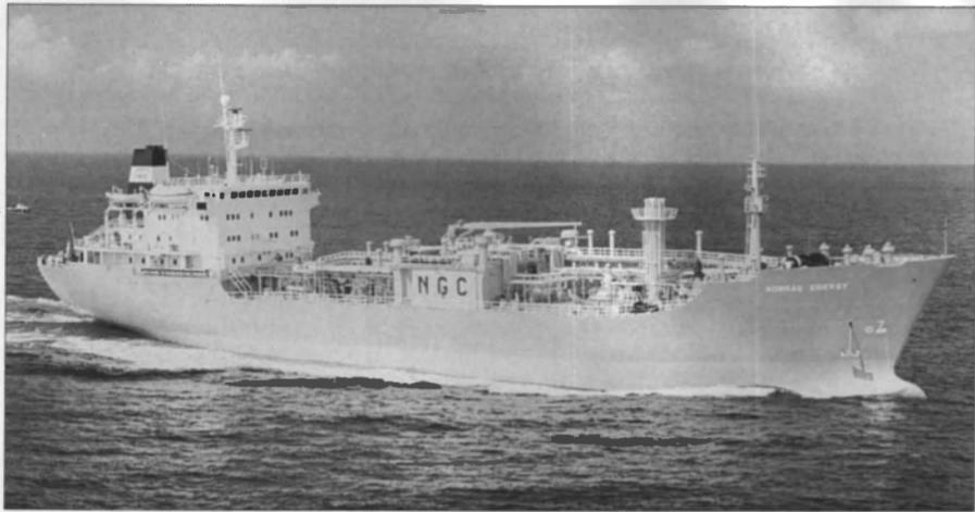
The LPG tanker Norgas Energy which was fitted with a new Wartsila Vasa 7R46 main engine.
