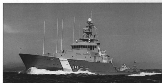
The Type "500" cutters are equipped with a Fume passive roll stabilization tank, mounted just below and forward of the bridge to significantly reduce roll amplitude in the severe weather conditions in which the cutters must operate. Maneuverability is aided by a 500-hp tunnel-type bow thruster.
