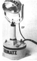
The Pesch SEEMATZ marine searchlights are constructed of seawaterproof aluminium and have extra hardened bi-vernal safety front panes. Servicing is facilitated by easy removal of the complete light unit from the rear. Light sources include halogen, xenon, high pressure mercury, metal halide vapour and tin halide. Available as hand-held, deck mounted, wheel-house control or remote control.
