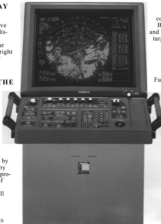
On-screen data readouts include range, bearing, course, speed, CPA, TCPA, BCR (bow crossing range), and BCT for up to 3 selected targets, as well as own ship course and speed.
