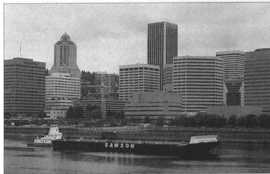
**FAIRWEATHER FOR SAILING**—Zidell Marine Corporation recently launched the Fairweather, a 1,600-ton deck cargo barge. The 302-by-76-by-20-foot Fairweather is the largest barge ever constructed at Zidell's Portland, Ore., facility. She will be operated by Samson Tug & Barge of Sitka, Alaska. Photo: Hugh Ackroyd
