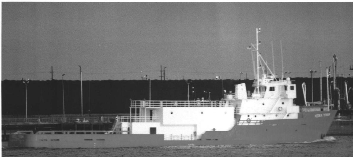
Steiner Shipyard, Inc. has completed the conversion of a 180-foot oil field supply boat Veesea Typhoon into a standby/rescue vessel for use in the U.K. sector of the North Sea. She is one of four standby/rescue vessels that will be operated by a joint venture between Vector Offshore, an English firm, and Seacor Marine, Inc. of Morgan City, La.
