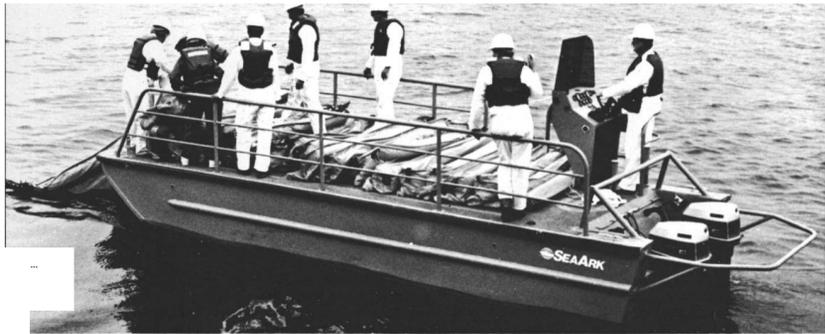
For immediate response to emergency spills, SeaArk's Model 2408-B Oil Boom Deployment Vessel can attain speeds of 44 MHP (38 Knots). Capable of carrying 1000 feet (304.8m) of 18 inch (.46m) boom, the need for timely and costly boat house boom storage is virtually eliminated. Shallow draft, ruggedness and dependability are just a few of the features provided by SeaArk's Transporter series. Call today for more information on all of our oil spill response products.
