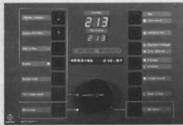
Besides indicating the actual position on a sea chart, the NAUTOPILOT offers, in systemtechnical combination with the adaptive autopilot NAUTOPILOT A, the track controller NAUTOTRACK and optionally a Nautical Information Display, the function of a track control system. Modern sea-going ships, such as the "Ship of the Future" utilize this technological advance.
