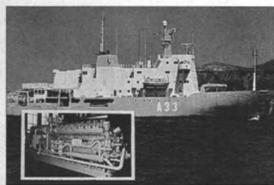
Four generating sets, two of them driven by 1,400-kw 14V 20/27 Bazan-MAN B&W engines (in the picture) and two by 7L 20/27 engines, are the prime movers for the diesel-electric propulsion plant of ocean research ship Hesperides.
