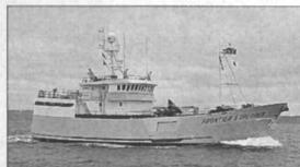
The Frontier Explorer, shown undergoing sea trials in Puget Sound following completion by her designers and builders, is based on Marco's successful MarcoMatic automatic longline system and a vessel with the proven ability to meet the needs of North Pacific longlining.
