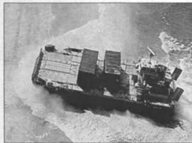
Built by Textron Marine Systems, LACV-30s accommodate a wide variety of payloads and can be disassembled for transport by truck, rail, aircraft or ship.
