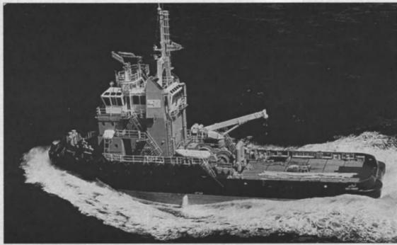
The superstructure of the Caterpillar-powered Hamour is placed well forward to create a large work deck aft and sufficient space for the towing/anchor handling winch.
