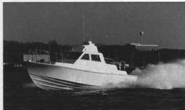
The Interdictor is available in lengths between 32 and 40 feet. Designed for launching at sea from a larger ship, the boats cruise at 30 knots with a maximum speed in excess of 35 knots. Beam is 11 feet 8 inches and draft is only 23 inches.
