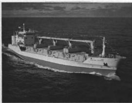
The vessel Erikson Crystal, showing high-speed Liebherr cranes of type CBW 5/19 Litronic, capable of working under offshore conditions.
