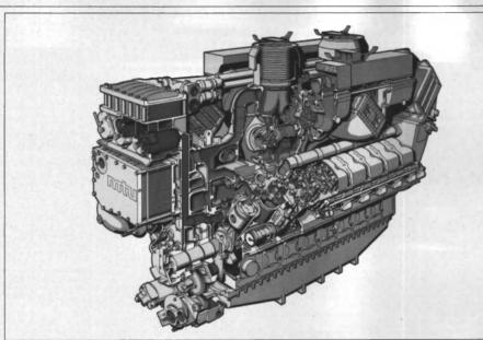
Cutaway drawing of the MTU 12-cylinder 595 TE50 engine.
