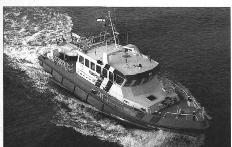
The police surveillance launch RP 9, built by Damen Shipyards, is capable of coming alongside ships with a dangerous cargo in accordance with ADNR appendix B (requirements valid for tankers).
