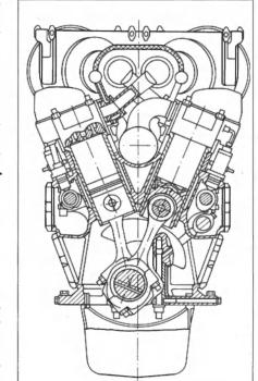
Schematic cross section of a V-engine of the new Deutz MWM series 632 (bore 240 mm, stroke 320 mm, maximum height about 2,550 mm).
