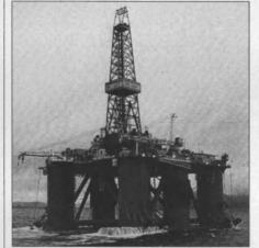
Foundations for two additional dual 100-hp tensioners are provided on the Drillmar I, along with space for additional tensioner air bottles, control panels, and riser joints should the owner desire to upgrade the unit for 2,000-foot water depth.
