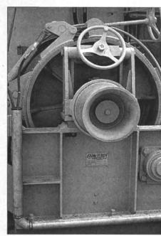
McElroy Machine & Manufacturing specially developed this winch for retrieving nets from waters as deep as 800 fathoms for Compagnie Francaise De Peche, a seafood processing plant in French Guyana.
