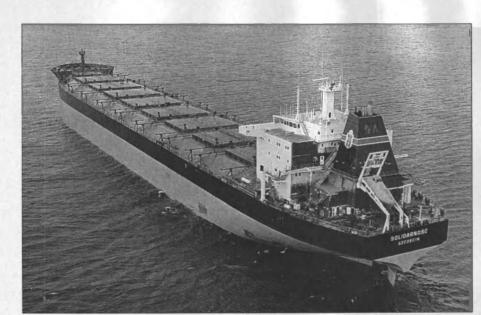
The bulk carrier Solidarnosc, recently delivered by B&W, features a new bow form which offers larger cargo volume and easier access to Hold No. 1, while maintaining the same performance standard.
