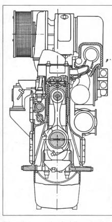
Schematic cross section of an in-line engine of the new Deutz MWM series 632 (bore 240 mm, stroke 320 mm, maximum height about 2,730 mm). Envisaged are in-line models with six, eight and nine cylinders.
