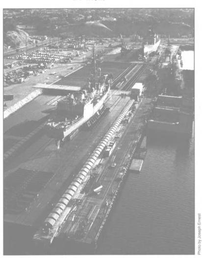
The highest capacity per metre shiplift in the world – 200 tons per metre for launching concrete caissons at Yunotsu, Japan.
