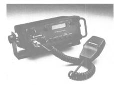
Harris's RF-3234 Remote Control Unit for the RF-3200 SSB radio.
