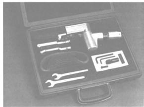
Dynabrade's new kit includes the tool itself, contact arm, and parts to quickly convert the Dynafile II to a die grinder or 2-inch disc sander.
