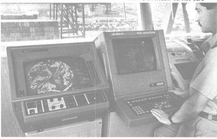
Crew member checks Raytheon Pathfinder ST/ ARPA and SNA-91 Bridge Integration display (right) at console of American President Lines C10 conbulk. In addition to interfacing with radar and other navigation equipment, the system interfaces with performance sensors to provide a wide range of important information in one spot, including navigation, engine, hull, and weather data.
