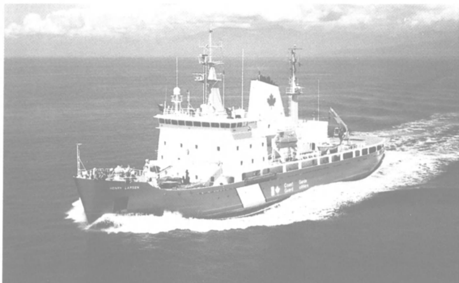
Versatile Pacific Shipyards Inc. delivered the Arctic Class 4 icebreaker Henry Larsen to the Canadian Coast Guard. Powered by an AC marine propulsion system that includes Wartsila Vasa diesel engines and General Electric Canada synchronous generators, the Henry Larsen can reach speeds of 13.5 knots in the open sea.
