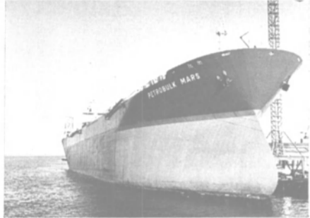
The 84,000-dwt product tanker Petrobulk Mars is the 10th in the series of product tankers of this type built by B&W since 1985.
