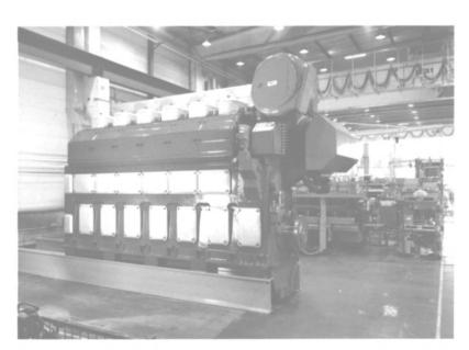
United Baltic Corporation's new RO/RO vessel will be equipped with Wartsila Vasa 46 main engines. Shown above is a six-cylinder version of the engine.
