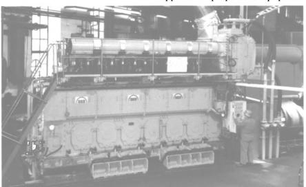
The diesel engine type shown. MAN B&W Diesel's 6L 40/54, will be used as part of a four-engine "father-and-son" power plant aboard a new Chandris cruise ship being built by Meyer Werft, Papenburg
