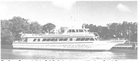
The Super Ranger, built by Gulf Craft, Inc., is powered by three Detroit Diesel engines, which produce a total of 2,160 shp at 2,300 rpm.
