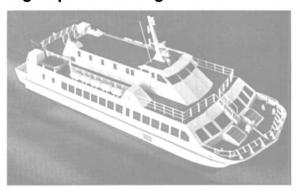
Model of the SES-Jetrider vessel. Two of this type of ship are being constructed in Sweden for use as high-speed passenger ferries
