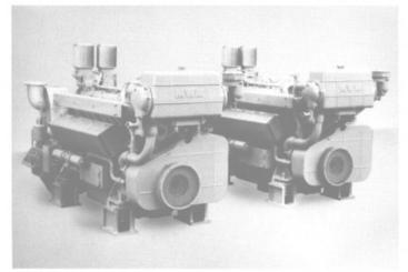
Twin TBD 234 V-12 diesel engines like these directly drive Riva Calzoni waterjets in a series of seven Spanish Customs patrol boats. The engines are rated at 1,000 hp each.
