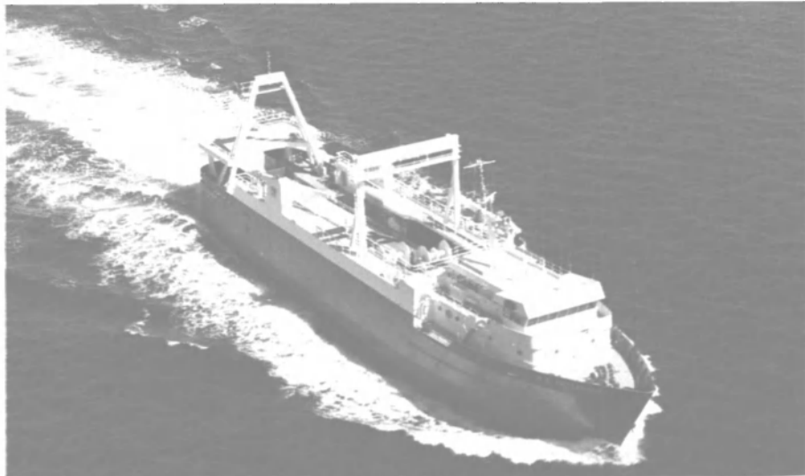
Powered by two Electro-Motive diesel engines, the U.S. Enterprise is the first American vessel designed and built to catch pollock and process surimi. She was built by Halter Marine, Inc.
