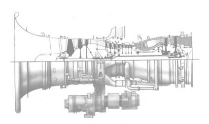
General Electric's LM1600 Simple Cycle Gas Generator.
