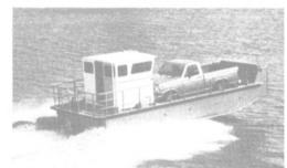
MonArk's 30-foot transportation barge is powered by twin AQAD40/290 Volvo I/O diesels (165 hp each).
