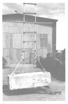
The ladder is shown above after completing the free-fall, when a 2,000-pound block of cement was attached to the lower step and hoisted clear of the ground.
