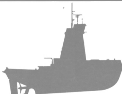
Artubar Tugs these 150 foot, 7,200 horsepower tugs are designed to connect with 5 deck articulated barges.
