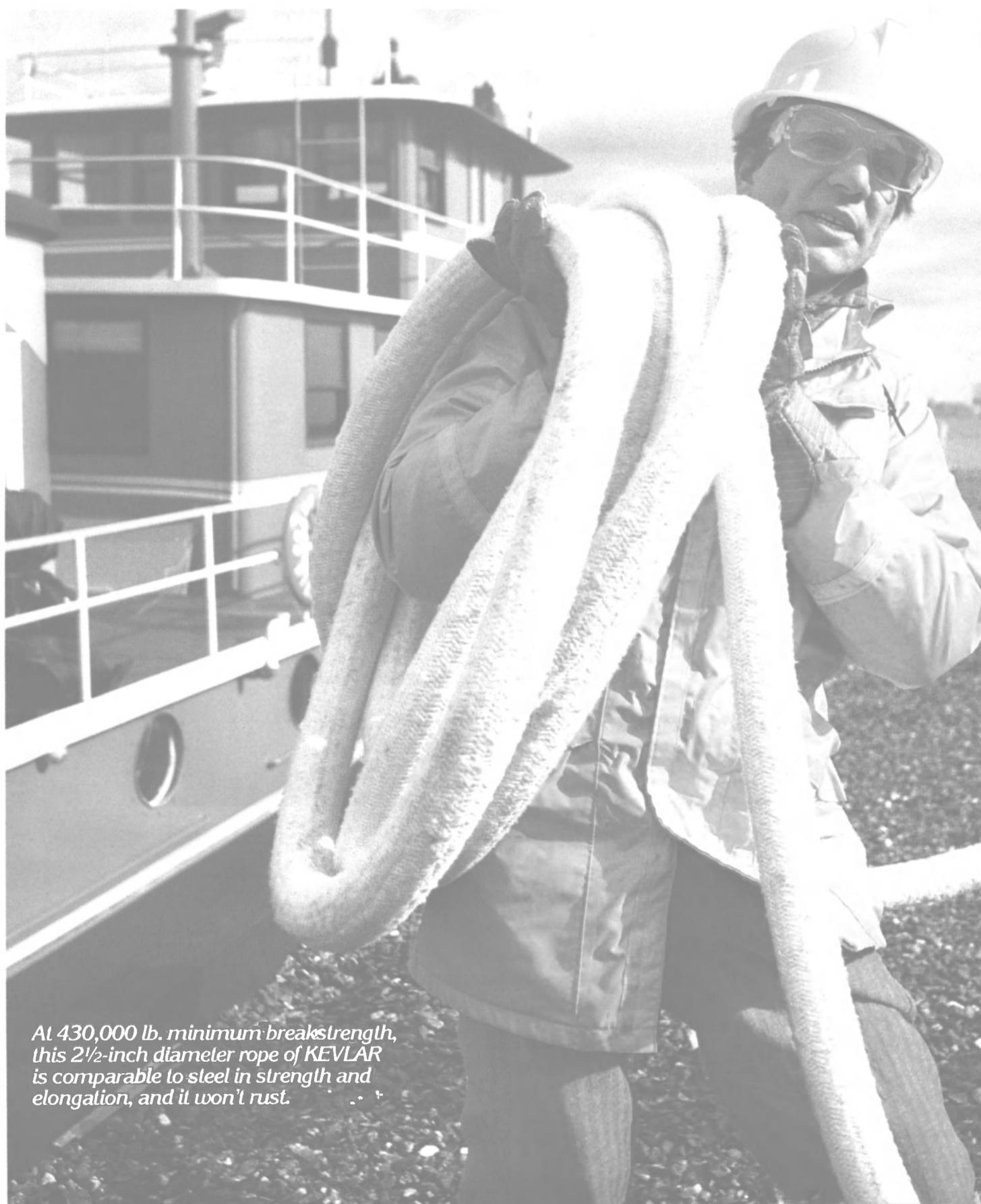
*At 430,000 lb. minimum break strength, this 2½-inch diameter rope of KEVLAR is comparable to steel in strength and elongation, and it won't rust.*
