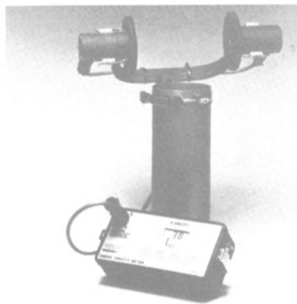
The Wager Model 650 is a new, portable diesel exhaust meter for use in checking, to air quality standards, the emissions of diesel-powered work boats, fishing vessels, barges, dredges, and offshore drill rigs.
