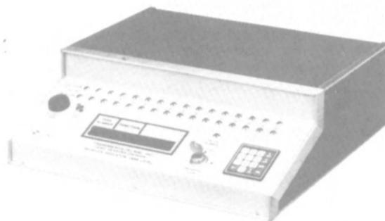
Gems Sensors Division, Plainville, Conn., recently introduced new microprocessor-controlled, desktop consoles for use with liquid level monitoring. These units can monitor 16 individual tanks on one panel and signal when alarm points have been reached.
