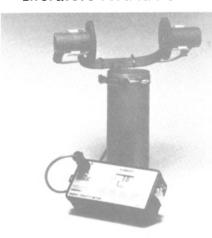
The Wager Model 650 is a new, portable diesel exhaust meter for use in checking, to air quality standards, the emissions of dieselpowered work boats, fishing vessels, barges, dredges, and offshore drill
