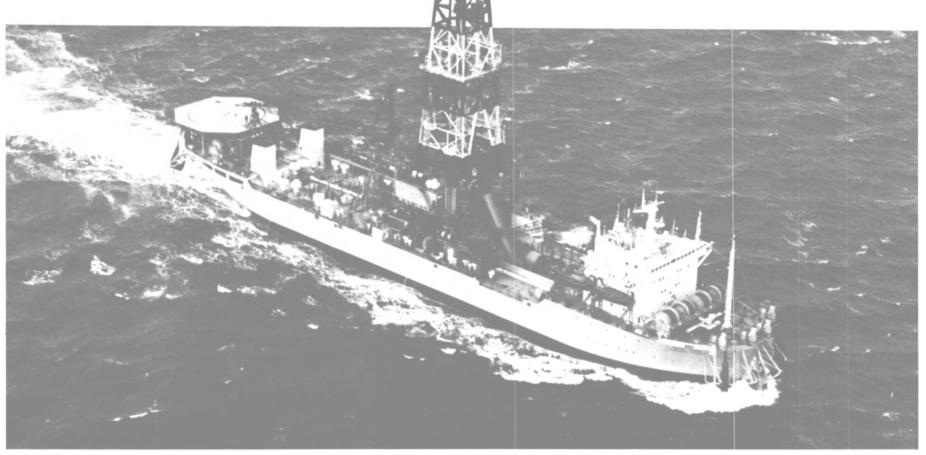
Building a drillship calls for a special blend of expertise. Which is why the Oil and Natural Gas Commission of India called on Hitachi Zosen to design and construct the SAGAR VIJAY — a self-propelled, anchor-moored drillship built under license of Gusto Engineering C.V., Holland.
