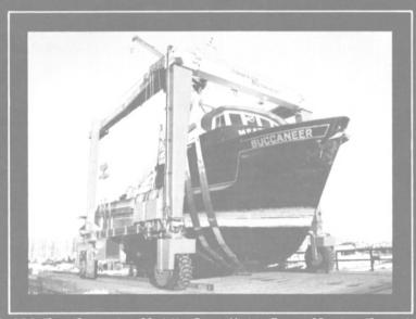
A 100 Ton Capacity Mobile Boat Hoist From Marine Travelift The Marine Travelift 100BFM is the newest addition to our complete line of mobile boat hoists. Marinas and boatyards around the world can take advantage of the "little" giant's versatility and be able to handle commercial fishing boats, work boats and pleasure crafts. The wide range of service means more customers and service means more customers and improved yard utilization.
