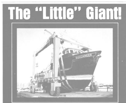
A 100 Ton Capacity Mobile Boat Hoist From Marine Travelift The Marine Travelift 100BFM is the newest addition to our complete line of mobile boat hoists. Marinas and boatyards around the world can take advantage of the "little" giant's versatility and be able to handle commercial fishing boats, work boats and pleasure crafts. The wide range of service means more customers and improved yard utilization.
