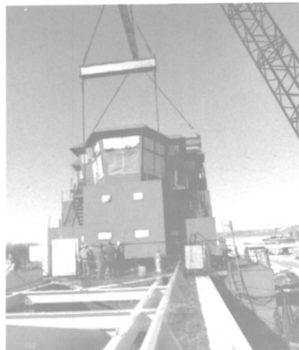
The pilothouse, shown above, just after being lifted in place on the Ouachita.
