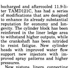
New pistons, liners, connecting rods, and turbocharger all contribute to the 121C's light-duty rating of 408 bhp at 2,000 rpm. Mediumand continuous-duty ratings are 387 bhp at 1,900 rpm and 367 bhp at 1,800 rpm. The engine uses 159 grams of fuel per bhp hour at the continuous rating.
