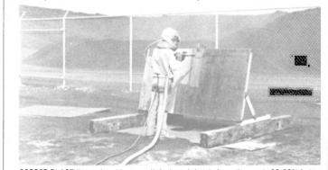
$\label{eq:copper} \begin{array}{l} \text{COPPER BLAST} (\text{in use here}) \text{ has very little dust, is low in free silica, cuts 30-50\% better than lower-quality slag abrasives and up to four times better than many silica sands. \end{array}$
