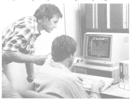
information logged by a TI 8000 Integrated Marine System installed on individual vessels, the system permits managers to download information to a Texas Instruments Professional Computer, and to apply advanced computer spreadsheet capabilities to the analysis of vessel operation.
