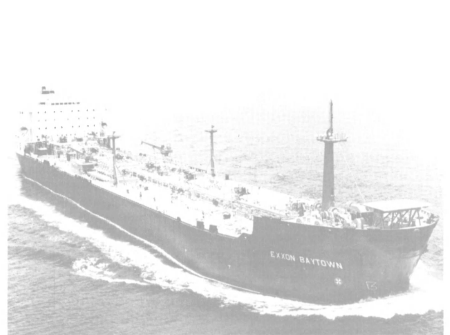
The 57,000-dwt Exxon Baytown, built by Avondale for Exxon Shipping, was christened and delivered recently. Crude oil carrier, built at cost of about $100 million, is powered by a slow-speed Mitsubishi/Sulzer diesel engine.
