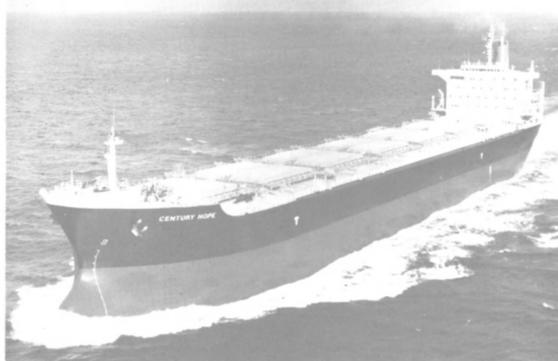
The 68,082-dwt bulk carrier Century Hope was recently delivered at the Tamano Works of MES to her owner, Kowin Shipping Company Limited of Hong Kong. Driven by a set of Mitsui-B&W 6L67GBE diesel engines she recorded a maximum trial speed of 16.32 knots.
