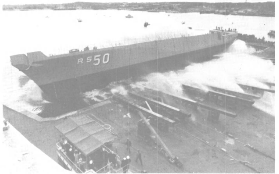
Side-launching of rescue/salvage vessel Safeguard (ARS-50) took place recently at Peterson Builders. She is first of four of a new class building at the Wisconsin yard.
