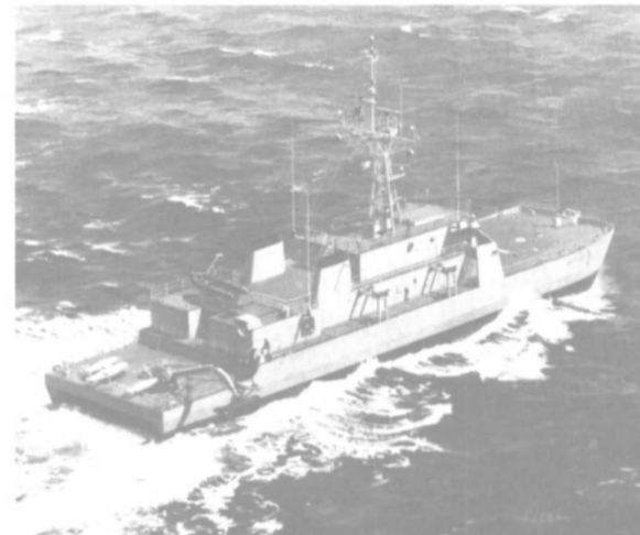
Artist's rendering of minesweeper hunter vessel that rides on a cushion of air. Bell Aerospace Textron is one of two companies participating in the final phase of the contract design and looks forward to participating in construction.
