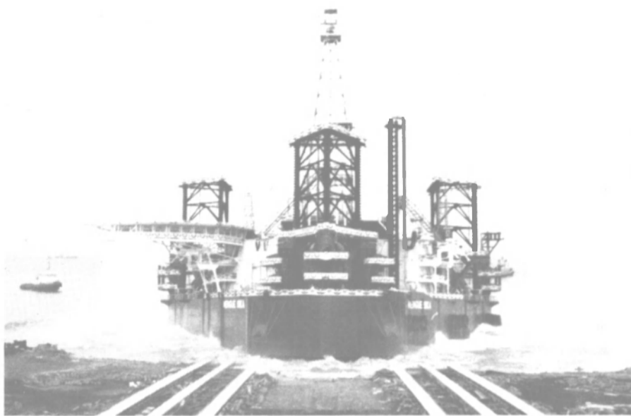
Jackup drilling rig Nengue Sika slides down the ways at recent Promet launch.
