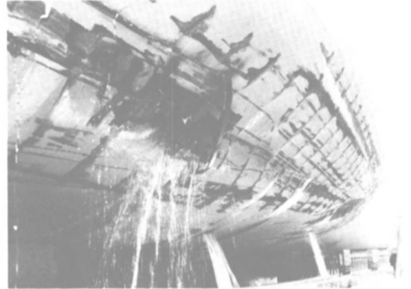
Hull damage to Strathetrick caused flooding of two holds.
