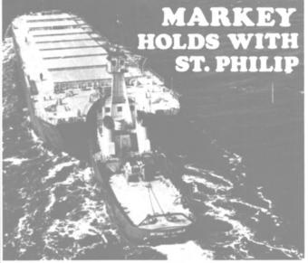
Tug ANTHONY P ST. PHILIP (and sister ALICE ST. PHILIP) are equipped with Markey Towing Winch, Capstans and Anchor windlass. These twin screw 5600 horsepower St. Philip tugs are engaged in regular cross U.S. Gulf service pushing 27,500 D.W.T., self discharge bulk cargo barges. St. Philip holds with Markey. Shouldn't you do the same?
