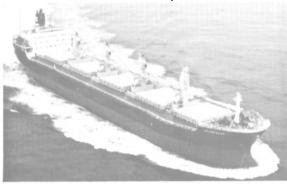
The Kepbreeze is a bulk-carrier powered by Mitsui B&W diesel engines giving her a full load service speed of  $14.8\ knots$ .
