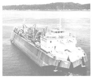
Unfolding, the split-hull self-propelled hopper barge Newport dumps its load.
