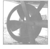
**MICHIGAN NOZZLE** SYSTEMS. When Michigan Nozzle Systems—which feature Kaplan-style bladesare compared to open props, they deliver more thrust with equal power, or comparable thrust with less power. Fuel savings have been reported up to 25%. **Bollard thrust increases** from 40% to 50% are also common. Thus, the logic for retrofitting with a Michigan Nozzle System becomes obvious: When operational costs go down, profits go up.
