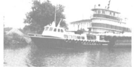
46' x 15' x 6' Aluminum Crewboat, Built 1981, Delta Bay Craft Shipyard, Twin GM 8-V-92 engines, 600 HP, 10 KW Generators, 28 Passenger, excellent condition.
