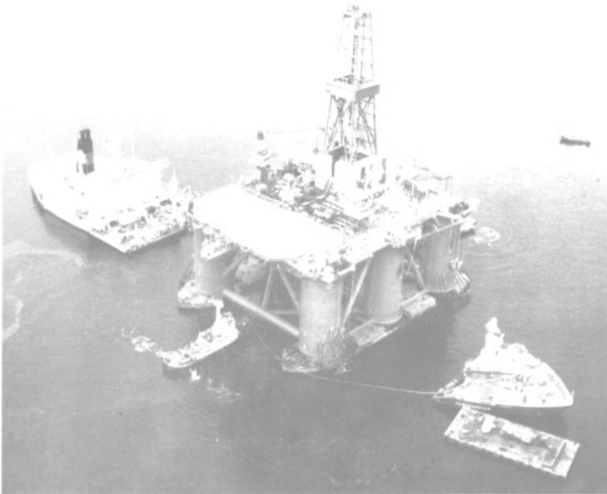
Drilling rig High Seas Driller, built by Daewoo Shipbuilding, being on-loaded aboard the heavy transport Ferncarrier.
