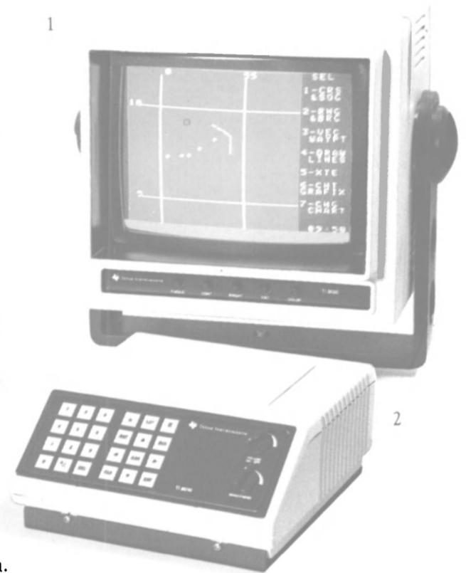
Three compact modules make up the TI8000: 1) Display Module—the size of a 10-inch television; 2) Command Module—a keyboard and cassette tape deck unit; and 3) Computer Module—8 × 10½ × 16 inches.
