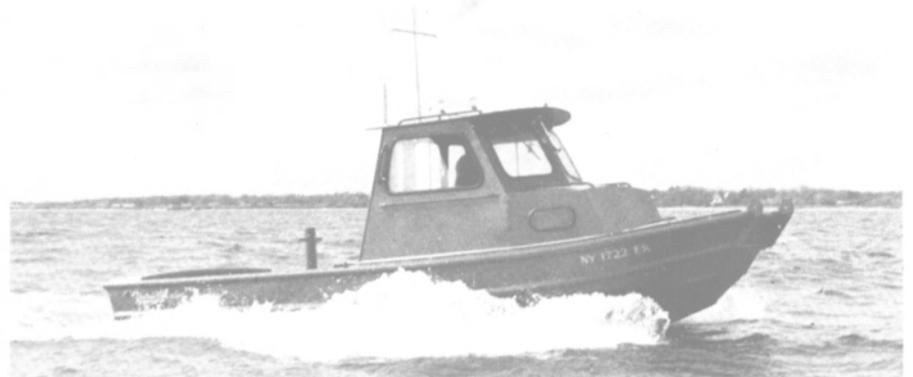
The Port Authority's new survey boat from Thomas Marine, Inc. is powered by a Perkins 85-hp diesel engine.
