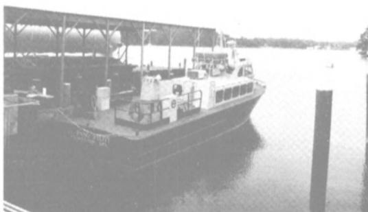
46' Crew Boat Aluminum Construction by Neuville Boat, 46' X 15' X 5' Twin GM 8V-71N 440 HP EA, 2:1 Reduction gear, 28 X 32 3 blade props, Keel Coolers, 7.5 KW gen, 30 passenger. Like New \$180,000
