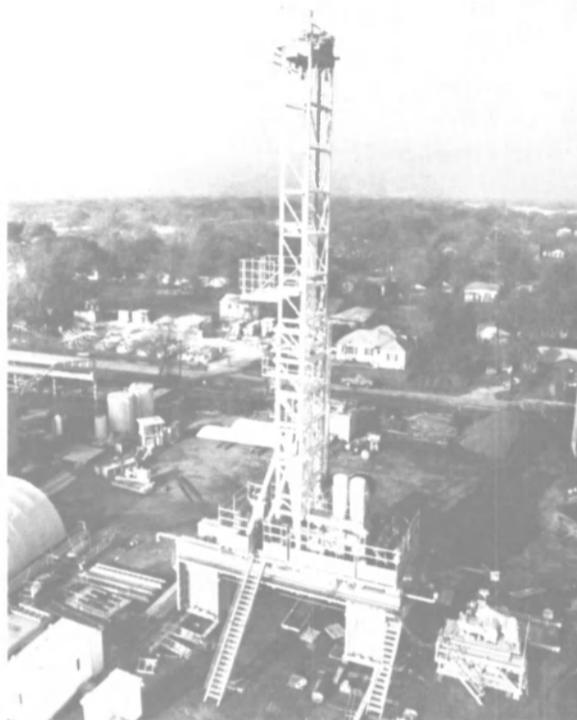
Hercules Workover/Drilling Platform Rig.
