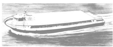
Artist's rendering of the 75-foot, 149-passenger commuter boat featuring a new hull construction process. The boat will be powered by twin GM 12V71 diesels.
