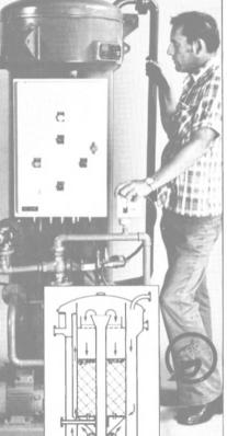
a pre-set degree of oil saturation, a very accurate vacuum-operated controller stops separation, initiates a cleansing back-flush cycle and
