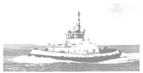
The tug Arthur Foss features a Voith-Schneider cycloidal propulsion system powered by two EMD diesel engines.
