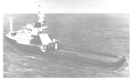
Model of the 235-foot-long ice-class offshore service vessel offered by Bender Shipbuilding.
