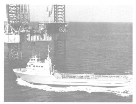
The Point Chaleur is powered by two EMD 16-645C diesel engines.
