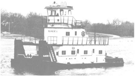
The Blanche V is powered by twin Cummins KTA-1150M diesel engines.
