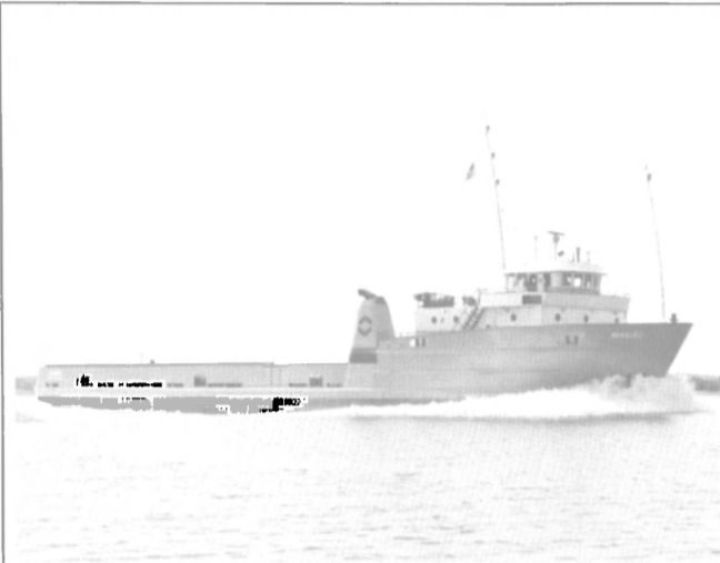
At work offshore for Petrobras is the Rincao, 185' by 38' with a 16' depth. This tug/supply vessel is one of five built for Brazil.
