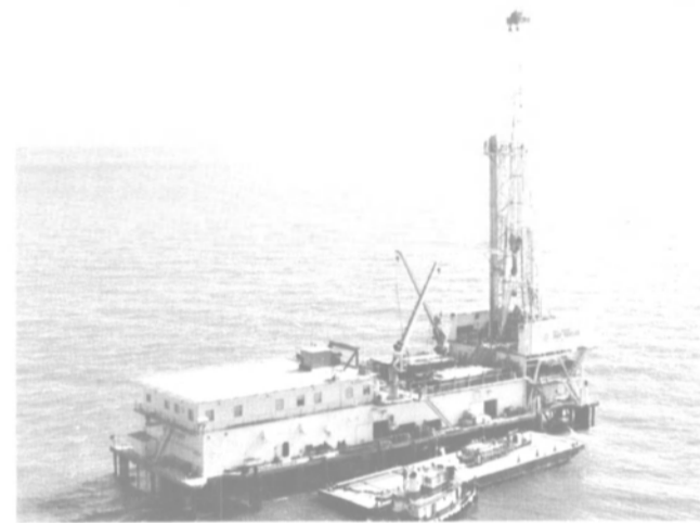
At work for the Louisiana based Circle Bar Drilling Company is the posted drill barge Pat Taylor. It is rated to work drilling depths of up to 30,000 feet.
