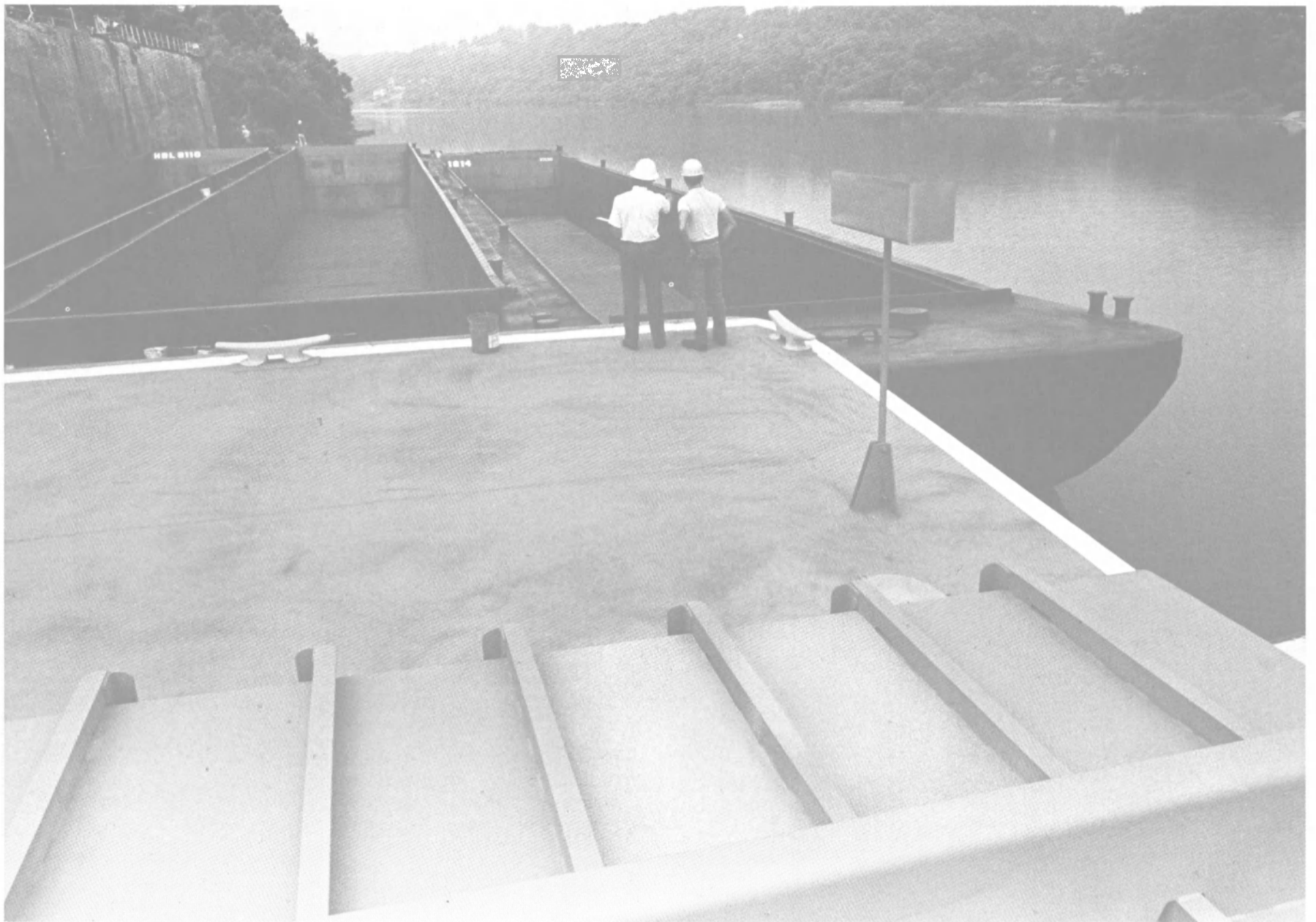
For two upriver coal customers with different operations: upper left, two 195 x 26 x 11 barges; right, a 175 x 26 x 11 barge; foreground, 195 x 35 x 12 hazardous cargo tank barge.
