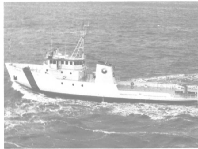
At work offshore for NASA is the UTC Freedom, 176' by 37'. Designed to recover the space shuttle's rocket booster, this vessel and her sister ship, the UTC Liberty, can also accommodate a variety of scientific and technical missions.
