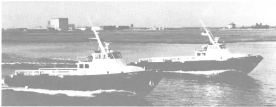
The Halter-built crewboats Pamela Ann and Patricia Ann are each powered by three Detroit Diesel 12V71TI engines.
