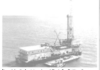
At work for the Louisiana based Circle Bar Drilling Company is the posted drill barge Pat Taylor. It is rated to work drilling depths of up to  $30,000\,\mathrm{feet}$ .
