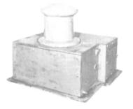
Totally enclosed 10 HP 440/3/60 1750 RPM motor. Barrell working area: top 111/2" diameter — bottom 13" diameter - over a 9" span. Deck space required 36" X 41". Total height 34".
