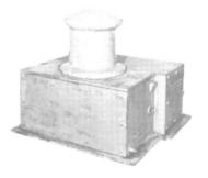
Totally enclosed 10 HP 440/3/60 1750 RPM motor. Barrell working area: top 111/2" diameter — bottom 13" diameter — over a 9" span. Deck space required 36" X 41". Total height 34".
