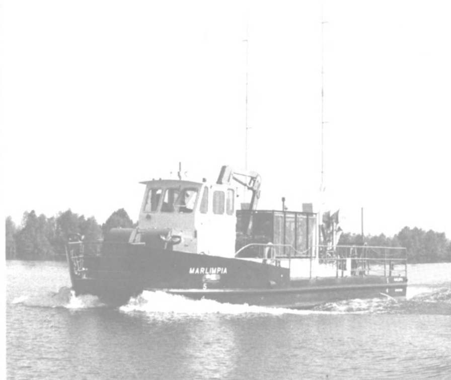
Two GM Detroit Diesel 6-71M engines power the oil recovery vessel Marlimpia. The oil recovery system was designed by Centrifugal Systems, Inc., of Houston, Texas, for use on Lake Maracaibo, Venezuela.
