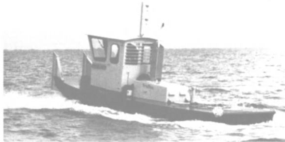
27 x 10 "Dredge Tender" built for Suffolk County Dept. Public Works 8,000 lbs. 140 hp. Detroit Diesel. 1/4" reinforced Plate Aluminum Push Knees add to the versatility. Two watertight bulkheads. 12 Knots
