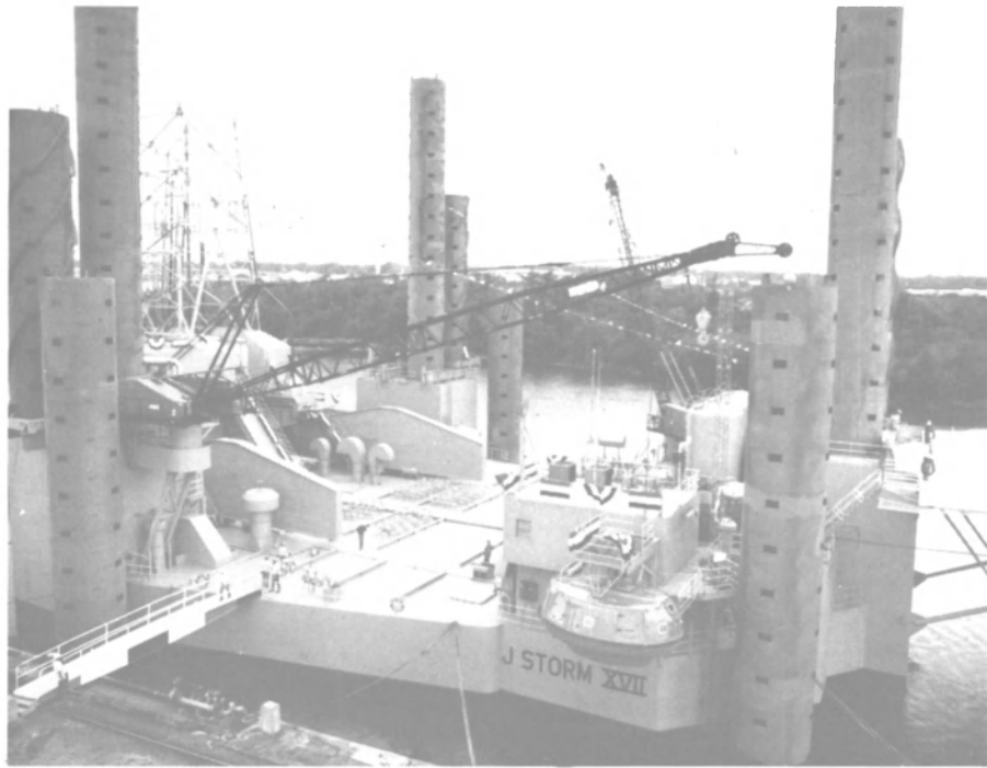
The jackup offshore mobile drilling unit J Storm XVII was the seventh rig completed this year by the Beaumont Yard of Bethlehem Steel.
