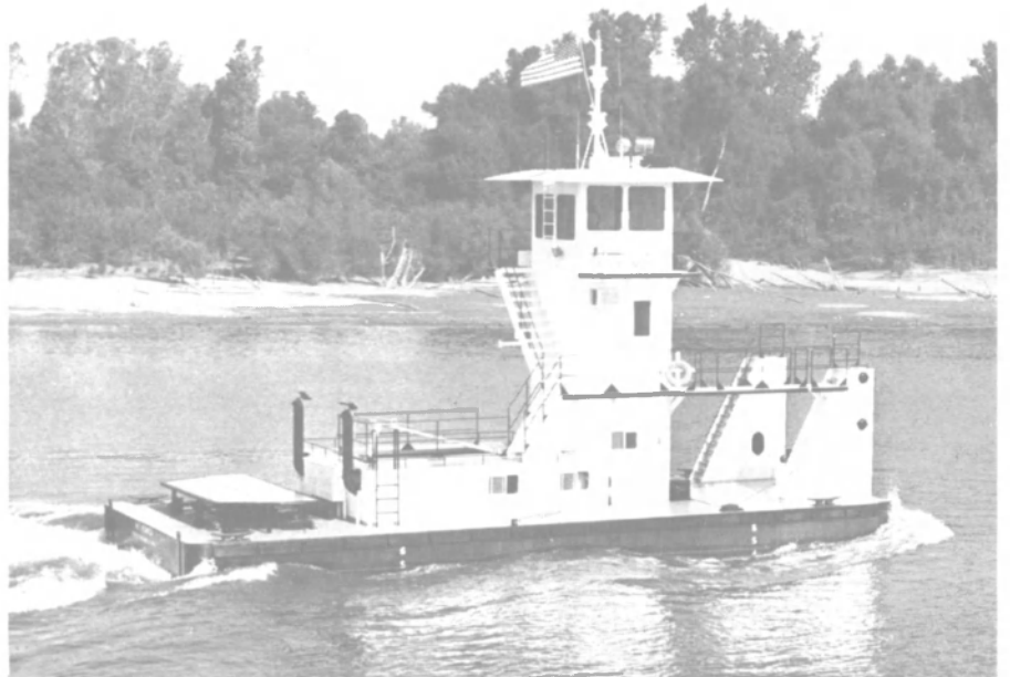
The towboat M/V Redneck is powered by two GM 16V-71 engines.
