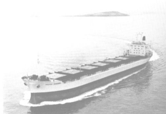
The Maersk Sebarok is the 47th Panamax-type bulk carrier built by Hitachi Zosen, Japan.
