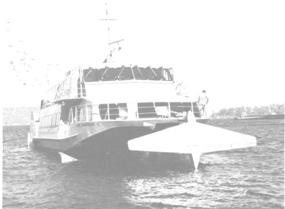
The Boeing jetfoil Bima Samudera I will be tested in a variety of assignments by the Indonesian government.
