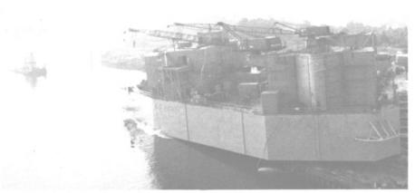
The Ed Holt, a Class 111-C self-elevating mobile offshore drilling unit, is launched at Levingston Shipbuilding Company, Orange, Texas.
