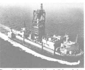
The world's first transportable polyethylene plant en route from Japan to Bahia Blanca, Argentina.
