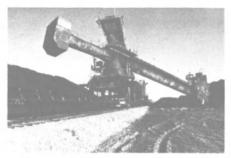
When marine equipment arrives to load coal at the terminal, the stacker/reclaimer picks up the coal at a rate of up to 4,700 tons per hour, delivering it to the barge loader.
