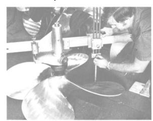
Michigan's Work-Horse<sup>TM</sup> is a tough 4-blade propeller with heavy cross-sections and heavy-duty leading edges designed to give you smoother operation than the 3-blade wheel it replaces. It is cast and available in three very strong materials: Michalloy K bronze and Ni-Bral through 30' dia., and CF 3 mod Stainless Steel in sizes through 18' dia. All offer exceptional resistance to corrosion and damage... could save costly haul-outs, repair and downtime.
