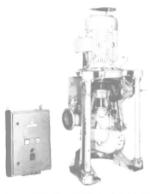
4" x 4" — 220 GPM @ 231' head (100 PSI) 1750 RPM (50M<sup>3</sup>/hr. @ 70M total head). Complete with vacuum pump. MOTOR: 25KW — 1800 RPM — 440/3/60Hz. Type 125-2VCS-A-NV. Teikoku Machinery Works, Osaka, Japan.
