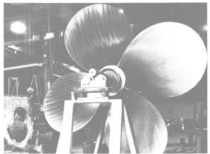
Coolidge Propellers have earned a world-wide reputation for tough, yet readily repairable stainless steel propellers. That's because, with more than 60 years of experience. Coolidge has accumulated vast knowledge about casting stainless steel. Coolidge also claims a world reputation for efficient prop designs. 3-, 4-, or s-blade styles up to 13' dia.. as well as CP blades, are available in bronze or stainless. Our engineers will create custom designs to suit your need.
