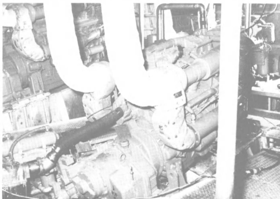
George Engine Co. of Harvey, La., modified the 12V93 TI engine for the five-screw crew/utility boat Joyce McCall II.
