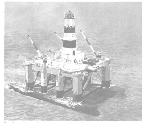
The Ocean Ranger II in an artist's rendition. The mobile drilling units will feature ship-shaped pontoons, ice-strengthened columns, and weather protection of drill floor and derrick.
