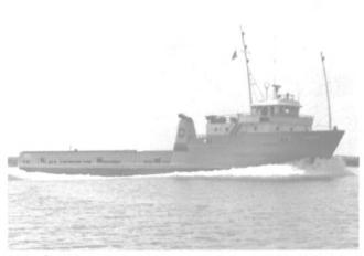
At work offshore for Petrobras is the Rincao, 185' by 38' with a 16' depth. This tug/supply vessel is one of five built for Brazil.
