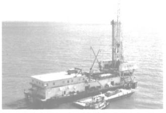
At work for the Louisiana based Circle Bar Drilling Company is the posted drill barge Pat Taylor. It is rated to work drilling depths of up to 30,000 feet.
