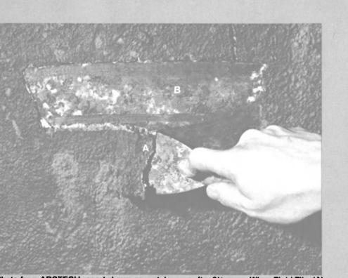
Photo from ABSTECH report shows no rust damage after 9½ years. When Fluid Film (A) was scraped away from ballast tanks, no oxidation was found on base metal (B).
