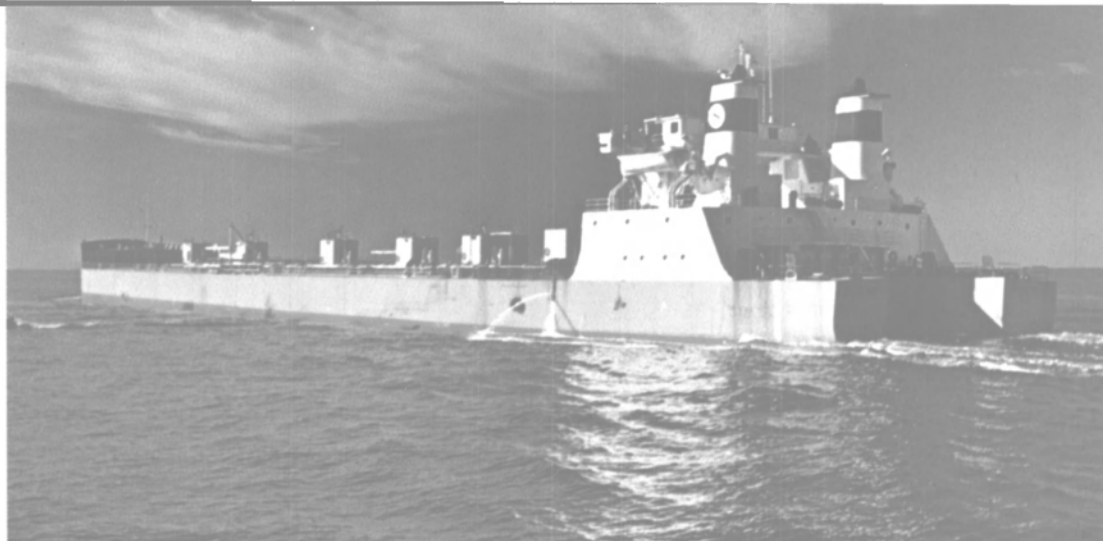
The M/V SEABULK MAGNACHEM, and her sister ship the M/V SEABULK CHALLENGER (above) are 39,000 ton integrated tug/barge combinations, transporting bulk liquids between U.S. Gulf and Atlantic Coast ports.
