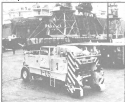
Deep-sea traffic by PAD Line in the Pacific. Straddle carriers supplied by Valmet.
